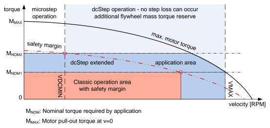
Safety margin: Classical application operation area is limited by a certain percentage of motor pull-out torque
