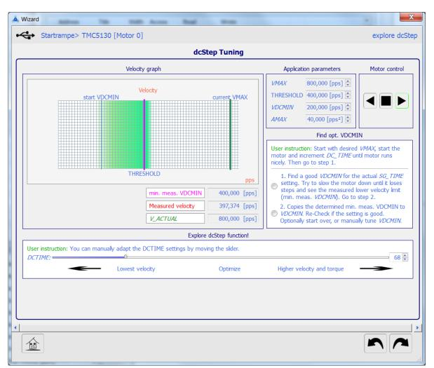
Now, start the motor by pressing the rotate right or rotate left button. Adapt AMAX if the motor cannot start up. If the motor does not accelerate when increasing *DCTIME*, decrease *VDCMIN*. In this case probably the motor already has reached the maximum dcStep velocity with the given current setting.
