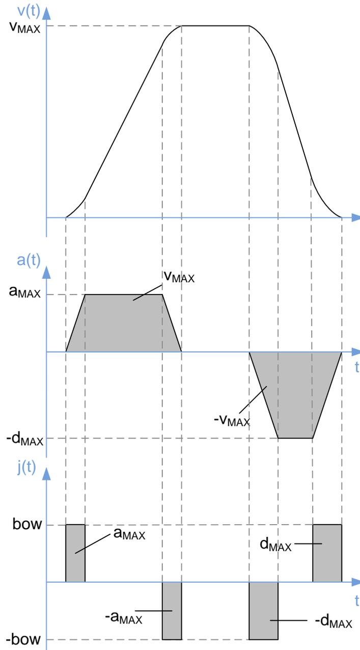
Figure 3 S-shaped velocity motion profile with linearly changed acceleration values and constant bow values (similar to the motion profile of TMC457 with  $bow\_max > 0$ )
