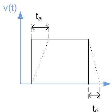
Figure 1 Constant velocity ramp (solid line) with real behavior of the system (dotted line)
