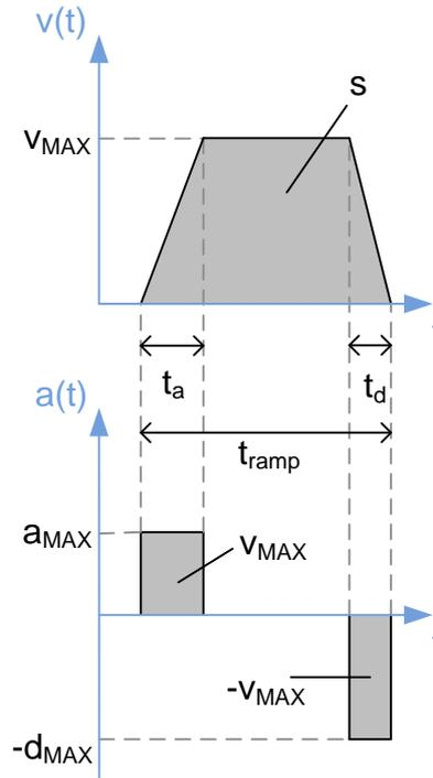
Figure 2 Trapezoidal velocity ramp with corresponding acceleration curve (similar to the motion profile of TMC457 with bow\_max = 0)
