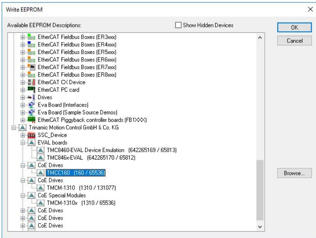
Figure 24: Selection of the TMCC160 device description
