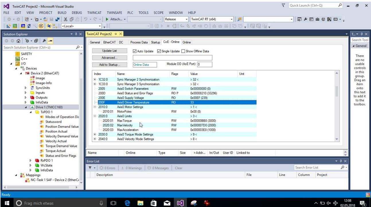
Figure 27: EtherCAT SDO Object: 0x200F - temperature
