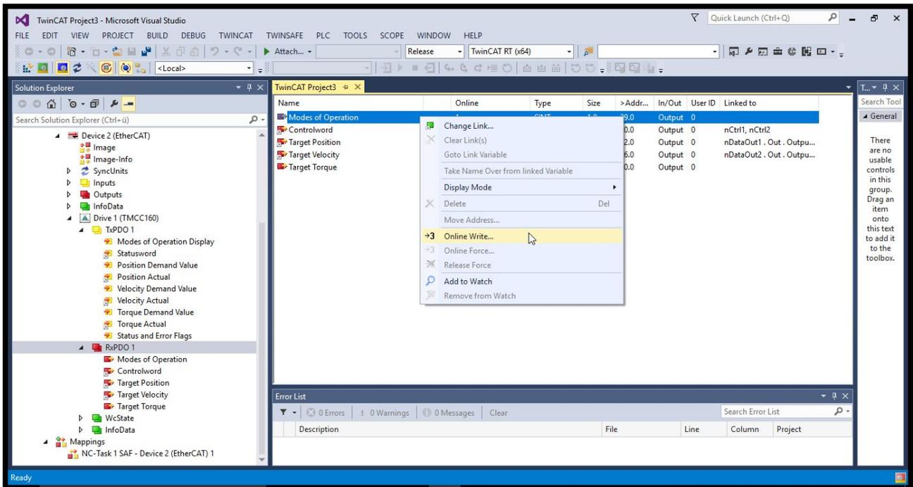
Figure 29: Write an Value to PDO
