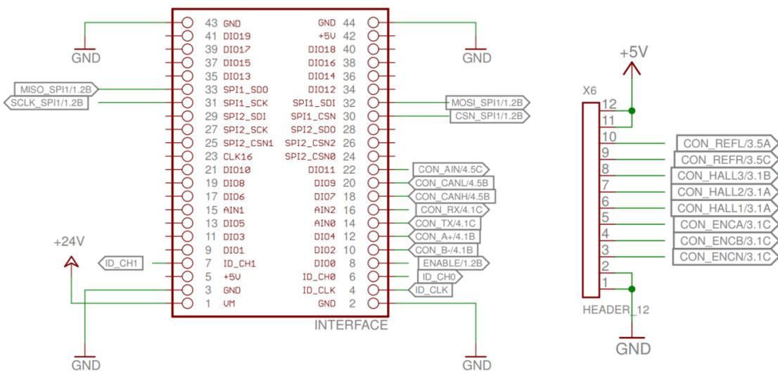
Figure 5: TMCC160-EVAL: Left connector and X6
