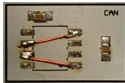
*Figure 1: Replacement of the CAN transceiver*
