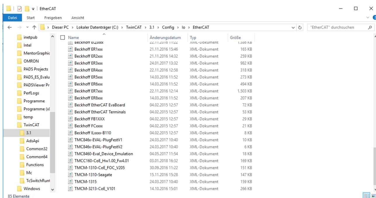
Figure 14: Copy the .xml to TwinCAT folder
