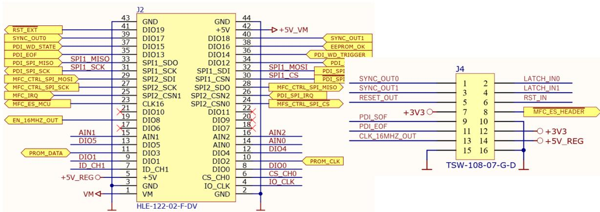
Figure 3: TMC8462-EVAL: Left connector and J4
