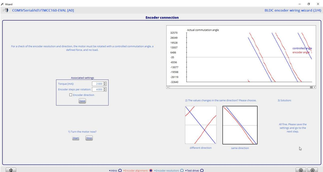
Figure 11: Encoder Wizard - Encoder alignment
