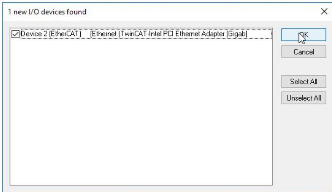
Figure 18: Found EtherCAT devices are displayed
