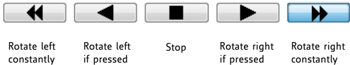
Figure 6.4 Jog tab keys for moving a motor
