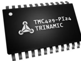
Figure 1: SOP24 example
