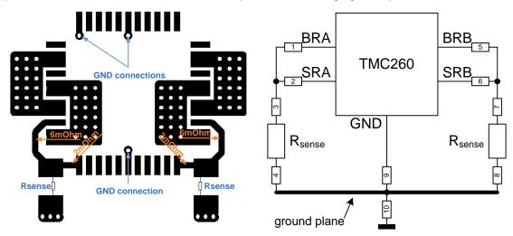
Figure 3: Example for a good layout (ground plane is not shown in the layout)
