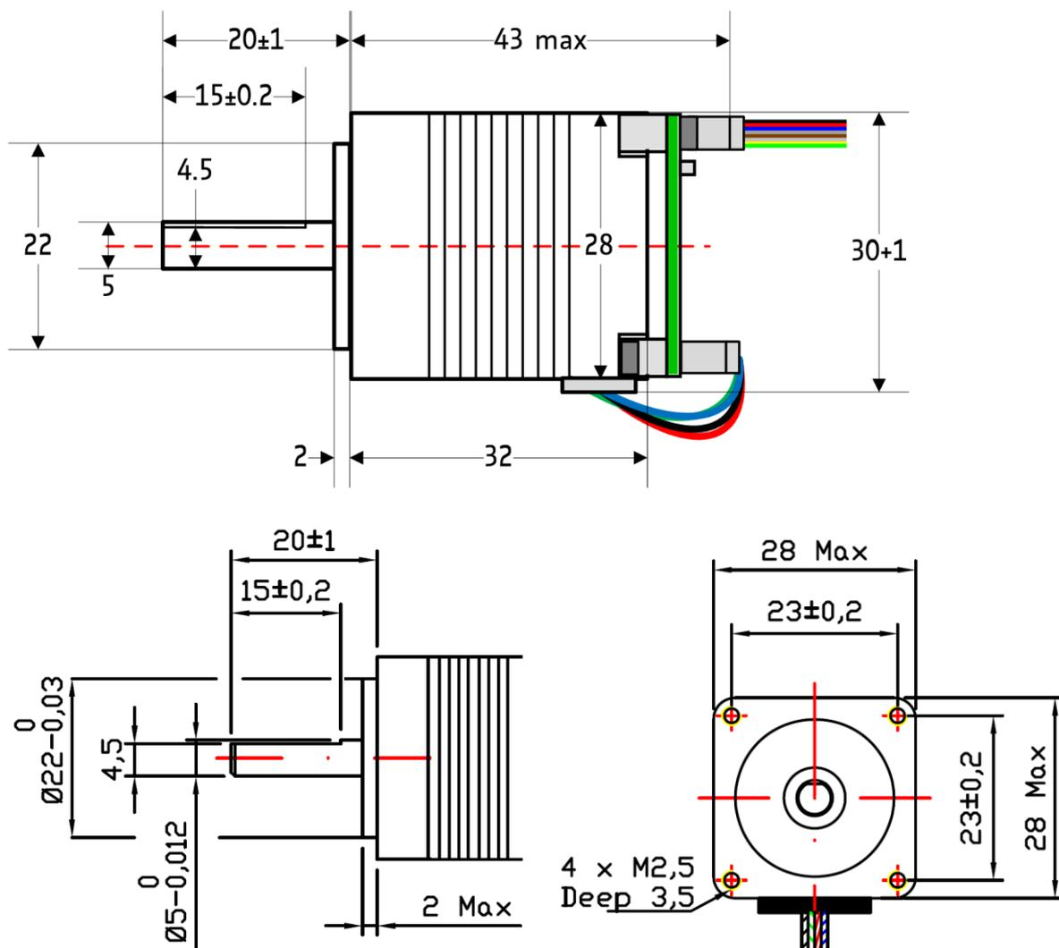
Figure 3.1 PD28-1-1021 dimensions (all dimensions in mm)
