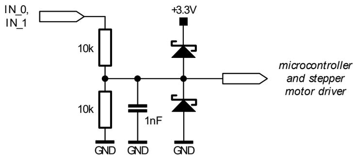
**Figure 3.7** General purpose inputs IN\_0 and IN\_1
