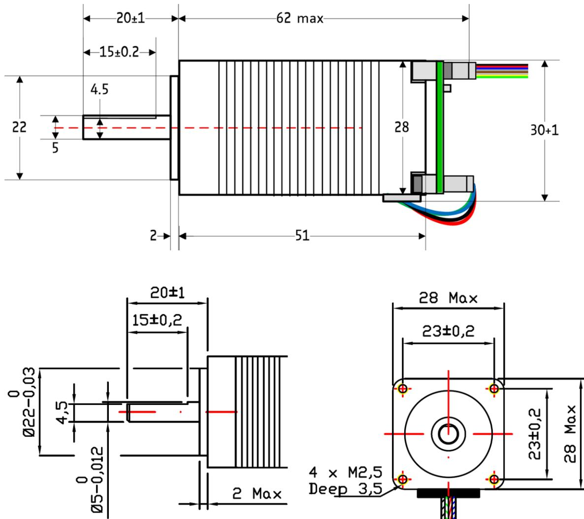
Figure 3.2 PD28-3-1021 dimensions (all dimensions in mm)
