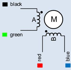
The diagram shows a motor symbol 'M' with two coils, A and B. Coil A has terminals labeled 'A' and 'A-'. Coil B has terminals labeled 'B' and 'B-'. Wires are color-coded: black (A), green (A-), red (B), and blue (B-). A legend indicates: black square for black, green square for green, red square for red, and blue square for blue.
