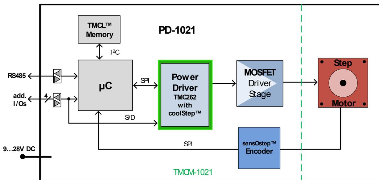
Figure 9.1: Main parts of PD28-1-1021 and PD28-3-1021
