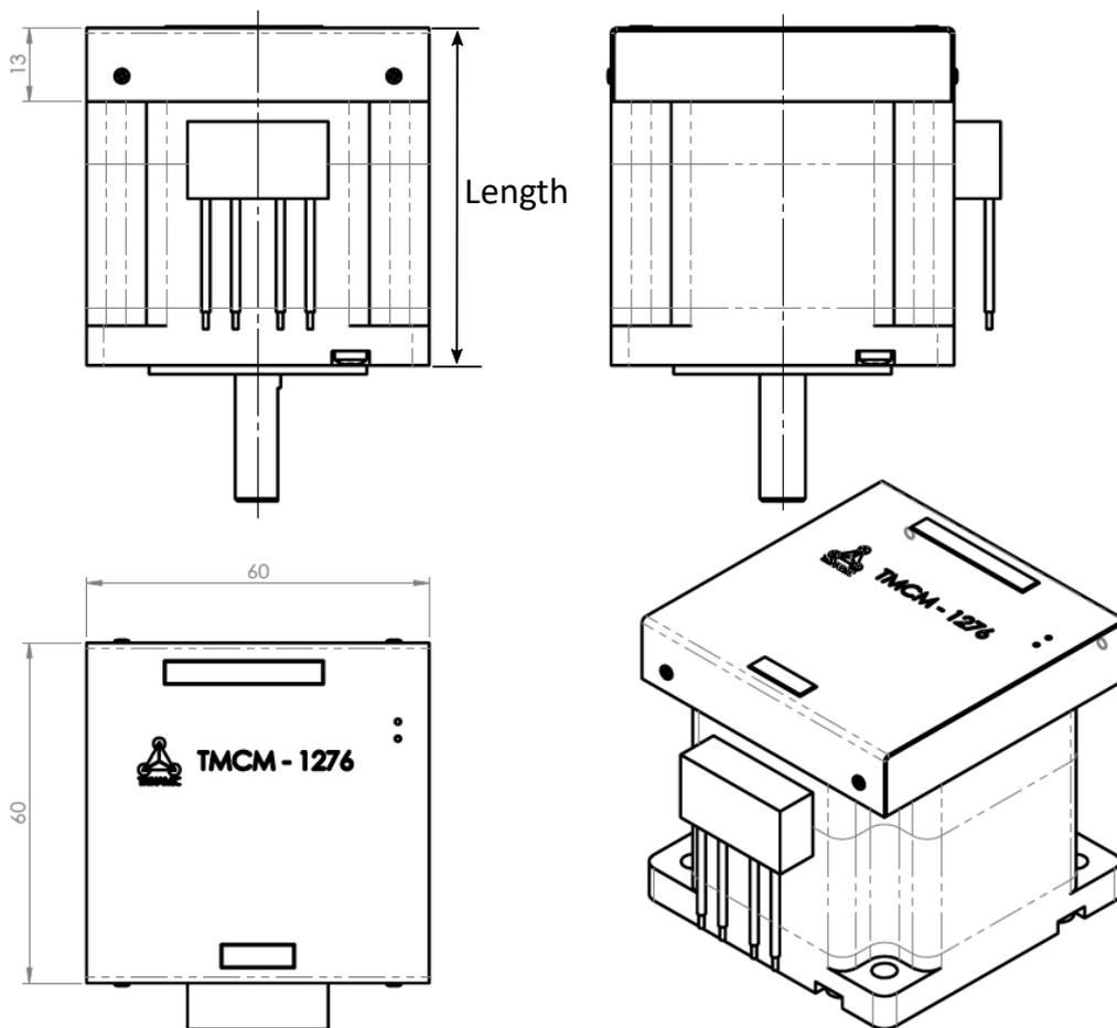
Figure 6: PD57/60-1276 all dimensions in mm
