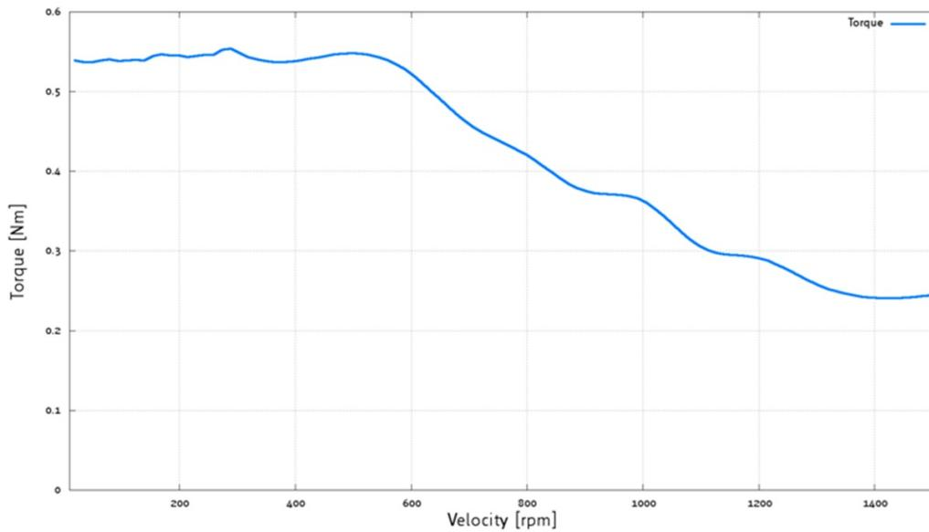
Figure 7: PD57-1-1276 torque vs. velocity 24V / 2.8A, 256µsteps
