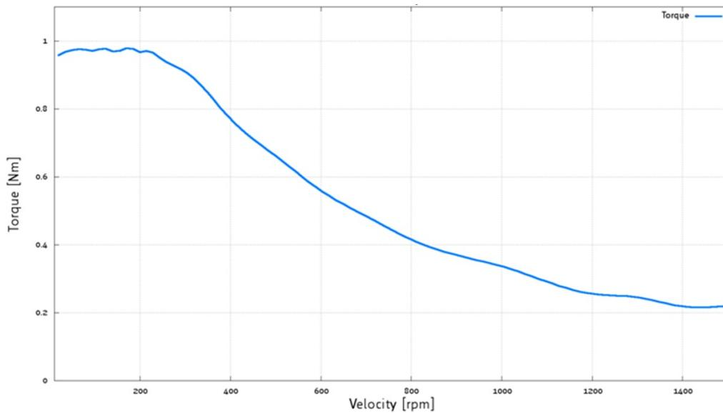
Figure 8: PD57-2-1276 torque vs. velocity 24V / 2.8A, 256µsteps
