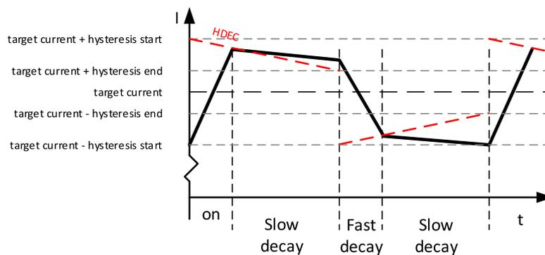
Figure 2: spreadCycle principle
