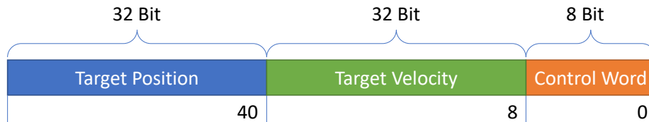
Figure 1: PD42-x-1243-IOLINK Output Process Data Bit Sizes and Bit Positions
