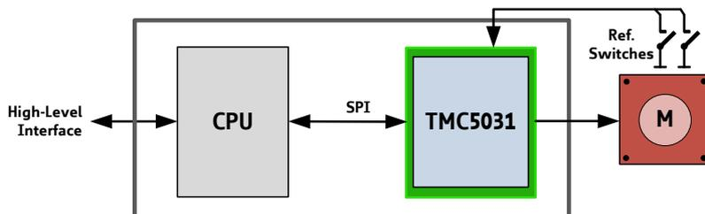
Two reference switch inputs can be used for each motor. A single CPU controls the whole system, which is highly economical and space saving.
