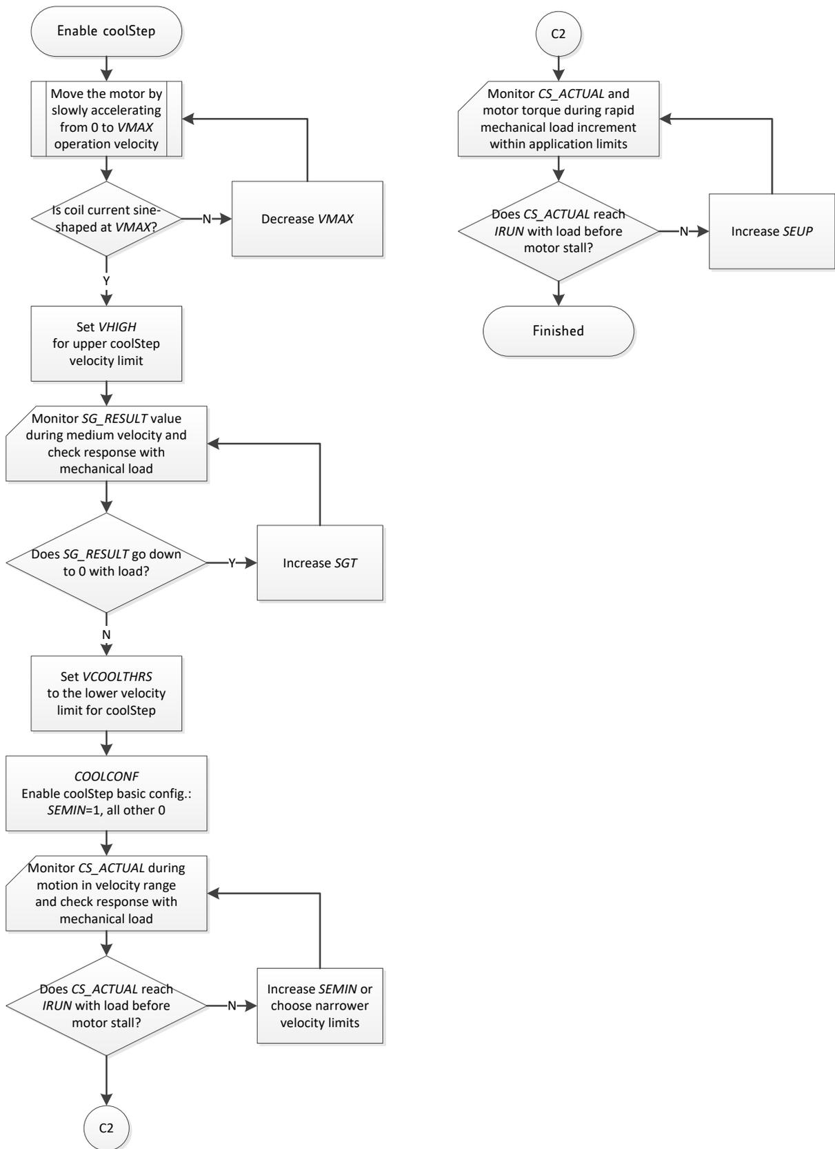
**Figure 13.3 Enabling coolStep (in combination with spreadCycle)**
