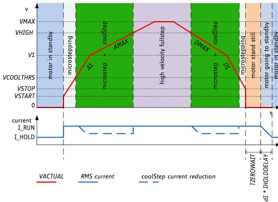
**Figure 9.3 Ramp generator velocity dependent motor control**
