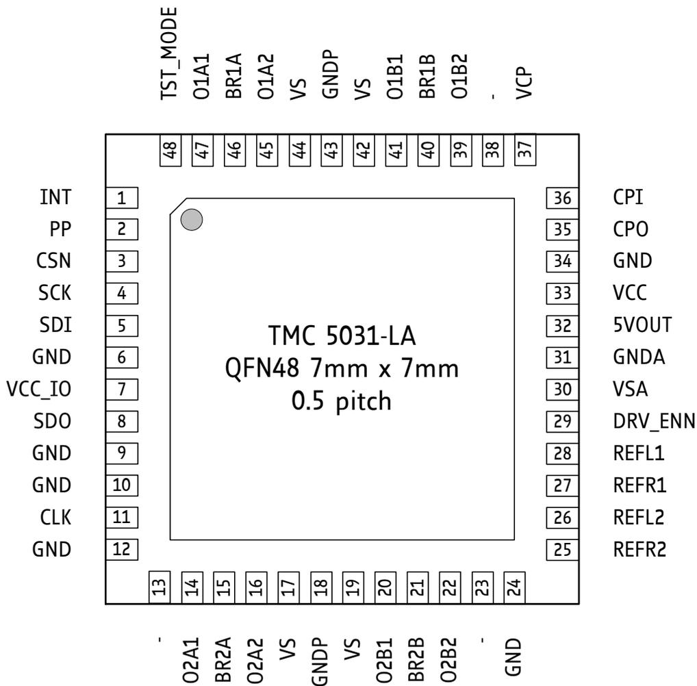
Figure 2.1 TMC5031 pin assignments.
