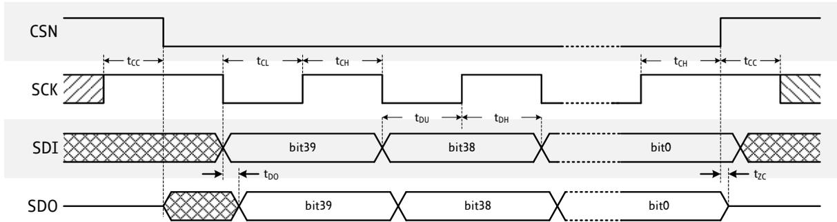
**Figure 4.1 SPI timing**
