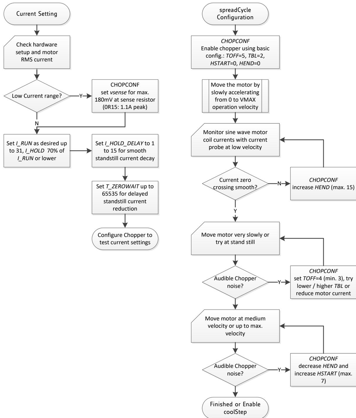
Figure 13.1 Current setting and setting up spreadCycle
