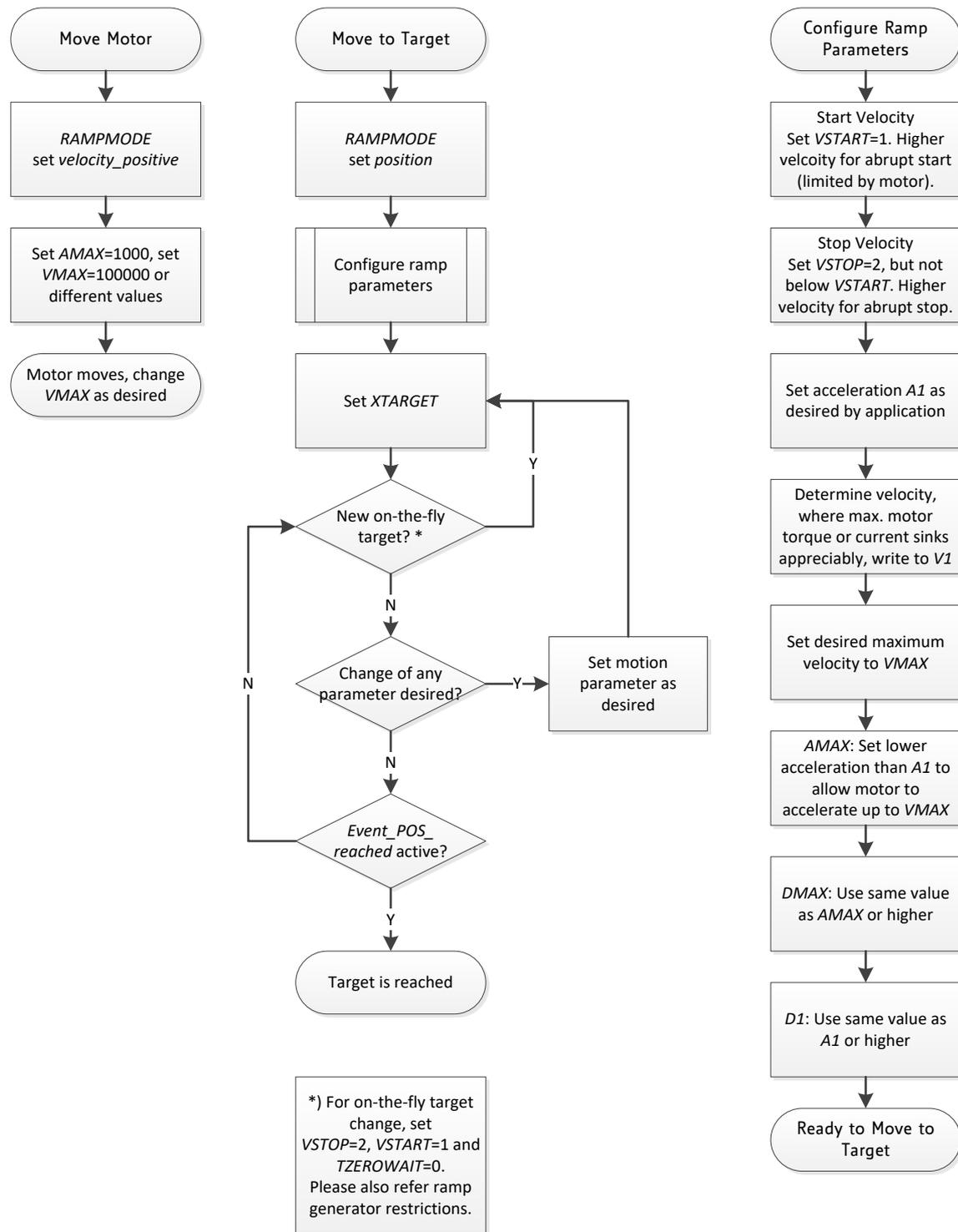
**Figure 13.2 Moving the motor using the motion controller**
