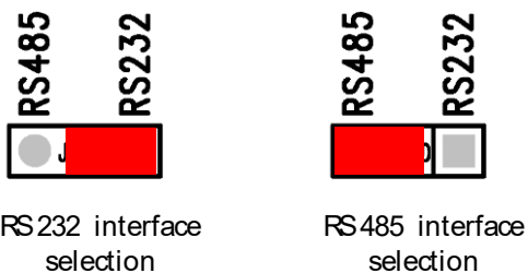
Figure 3.11 RS232/RS485 interface selection
