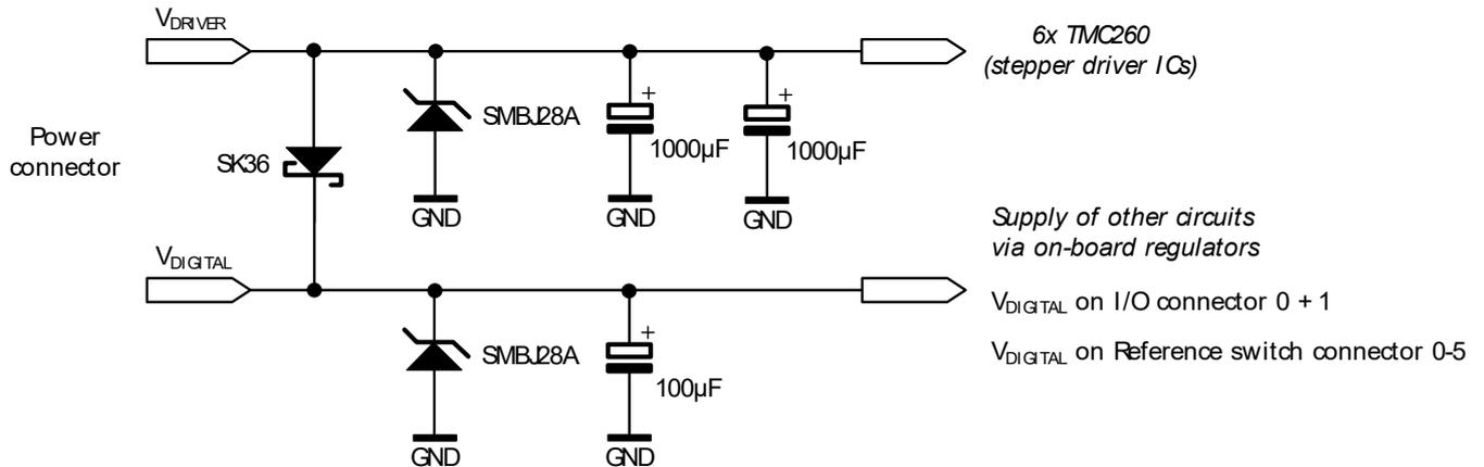
Figure 3.4 TMCM-6110 power supply concept
