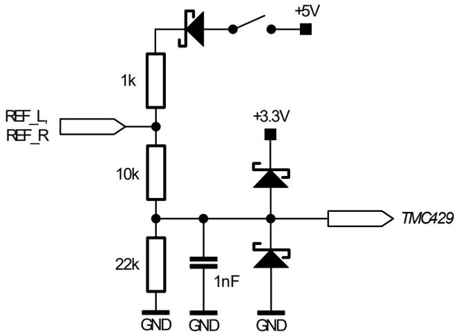
Figure 3.8 Reference switch input circuit (simplified diagram)
