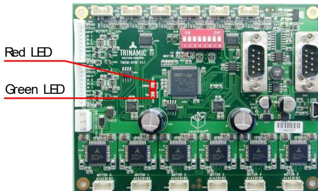
Figure 5.1 On-board LEDs
