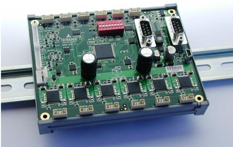
Figure 3.2 DIN rail mounting
