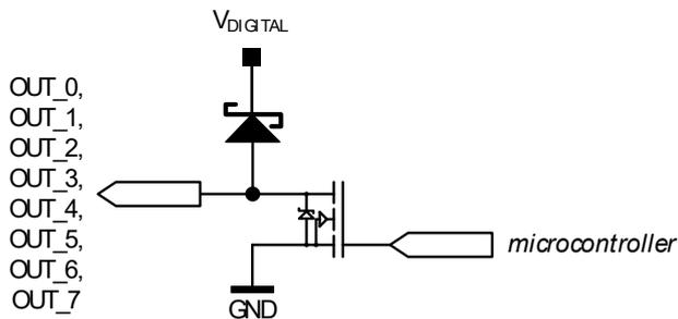
**Figure 3.11 General purpose output (open-drain with freewheeling diode)**
