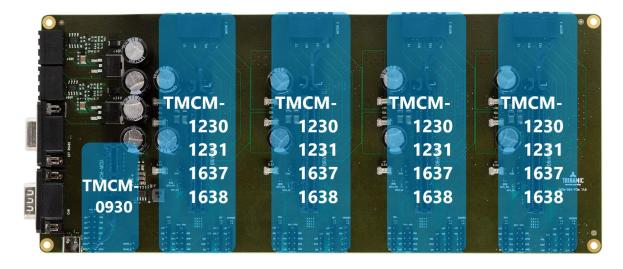
Figure 1: TMCM-BB4 Base board with available slots
