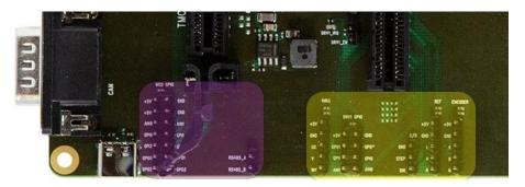
Figure 4: GPIO connectors of TMCM-BB4
