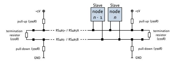
Or add resistor network at both ends of the bus (like Profibus<sup>™</sup> termination):
